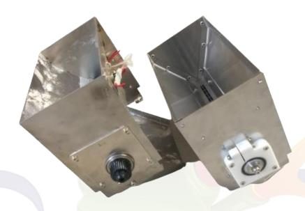
Picture 3: original unit on right hand side, redesigned unit on left hand side
